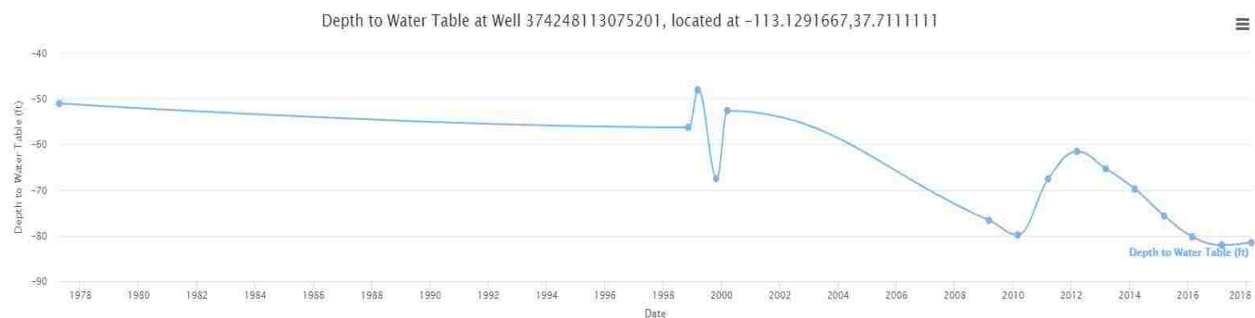
Figure 2-7: Inconsistent Sampling Rate at Well 374248113075201 near Cedar City, UT
